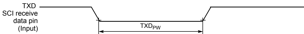
Figure 10-17 TXD Pulse Width
