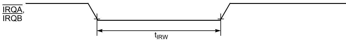
Figure 10-6 External Interrupt Timing (Negative Edge-Sensitive)
